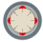
Refilling the tyre with atmospheric air actually accelerates the decay of tyre rubber, as the newly introduced oxygen attacks not yet broken double bonds deeper inside the casing, and closer towards the tread face.
