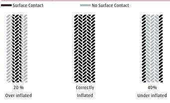
Many studies have shown that as much as 3 % - 5 % increase in fuel consumption and a remarkable high tyre tread wear is caused by to low tyre pressure.
