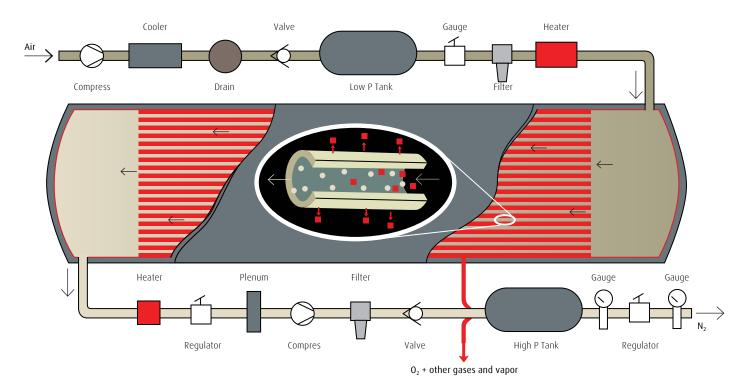
The process can be described as follows: Compressed dry air enters the cartridge on one end. Oxygen, other gases and rest humidity permeate faster than nitrogen through the membrane walls, thus enabling a side venting of those gases to the
