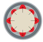
At some stage the outer tread face comes into contact with the degraded rubber layer. At this point, the durometer hardness of the rubber changes, and typically tread wear accelerates.
