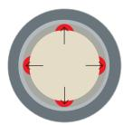
Once the antioxidants are filled, oxygen attacks the unsaturated double bonds in the rubber, from the inside of the casing outward. As oxygen breaks these double bonds, the tyre is continually losing pressure.
