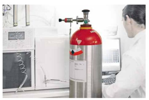
HiQ® gas mixture for Gas Chromatograph (GC) calibration
